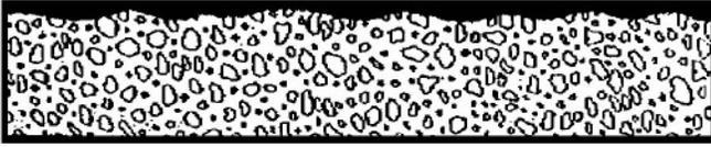
Cross-section of concrete showing contamination from laitance, efflorescence or atmospheric pollutants.
