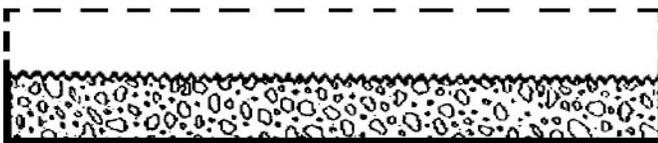
Cross-section of concrete after acid etching or rotary drum sander profiling.
