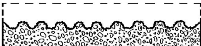
Cross-section of concrete after scarifying or mechanically scratching this surface.
