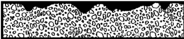
Cross-section of concrete showing contamination from substances such as oils, grease, wax, etc.
